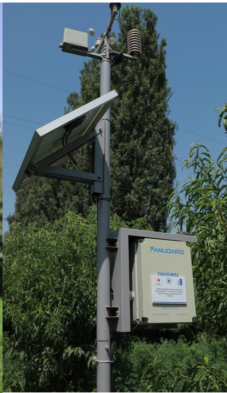
the agrometeo network in Fergana Valley and increase the coverage and forecast preciseness 40 small agrometeorological stations have been installed in Fergana Valley.
