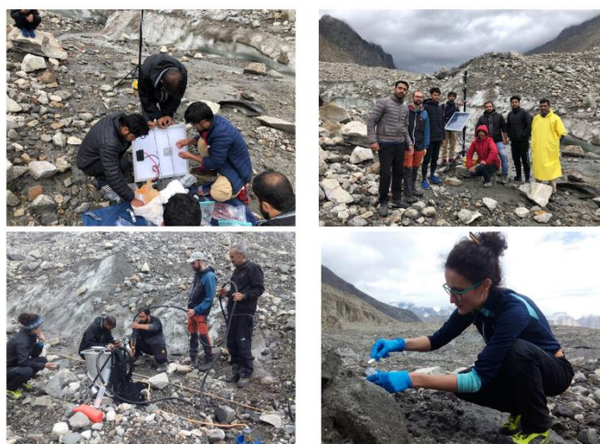
Figure 16: Field activities on Ghulkin glacier. From top left, clockwise: mounting of solar panel on temporary AWS; the AWS operational with the students from University of Baltistan and members of EPA-GB; drilling operations with the steam drill; sampling of debris for analysis of the plastisphere.
