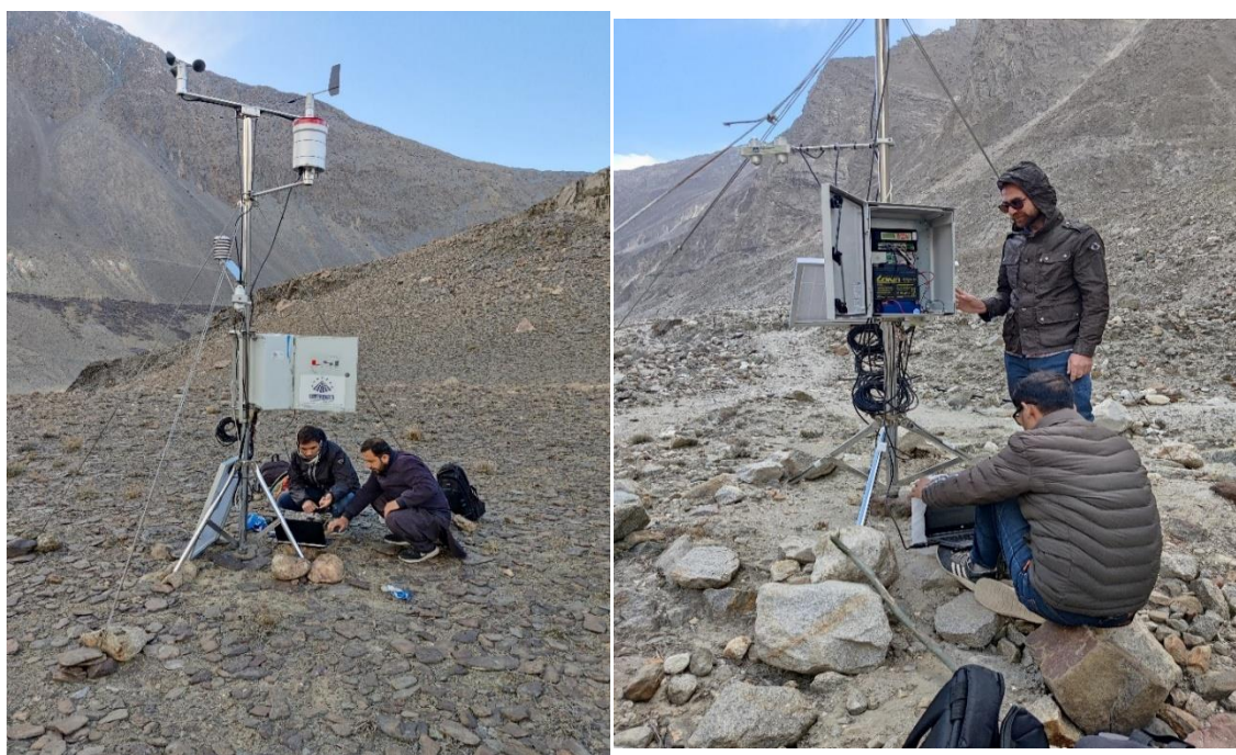
Figure 2: AWS installed at Shisper and Passu glacier
